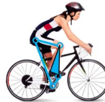
Fig.3. Cyclist's bicycle treated as a four-bar linkage
